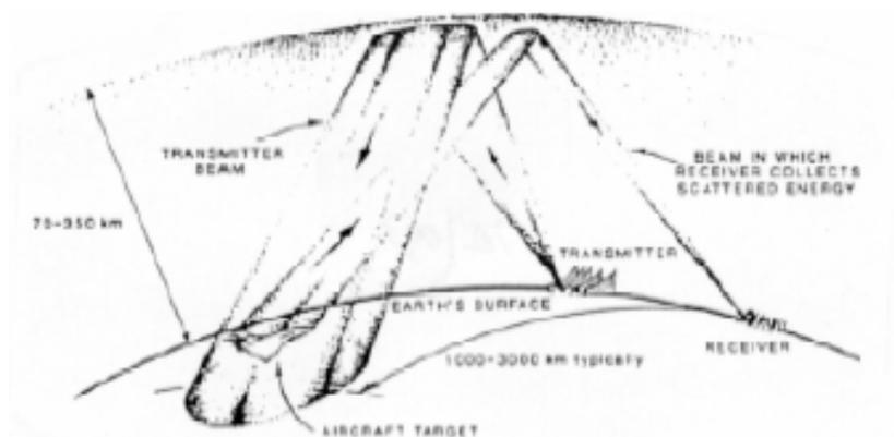
*Principle of Over-the-Horizon Radar*
