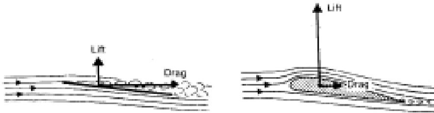
**4027.** Bernoulli's principle associates a decrease in Static Pressure with an increase in Velocity.
