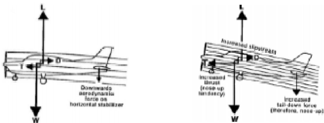
FIG 1.5. - INCREASING POWER CAUSES NOSE-UP TENDENCY
