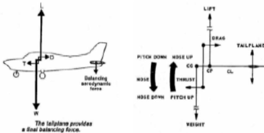
FIG. 1.3. - THE FOUR FORCES - THE FORCES IN BALANCE
