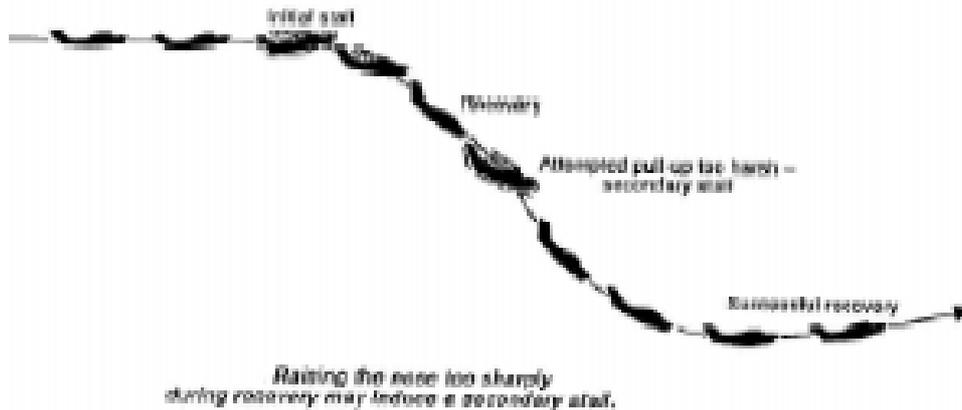
**1045.** During a stall, the flight controls are less effective due to reduced airflow. Use of the elevator and rudder are required. A symptom of a stall can be a **wing drop**, which, if tried to be corrected with opposite aileron, causes further drop on one wing than the other, and the aircraft can develop into a spin. To overcome the wing drop, opposite rudder is applied. This overcomes the yaw effect.
