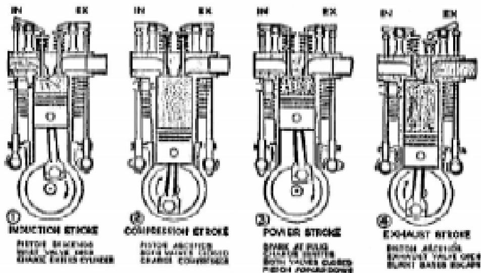
FIG 3.1. - THE FOUR STROKE CYCLE
