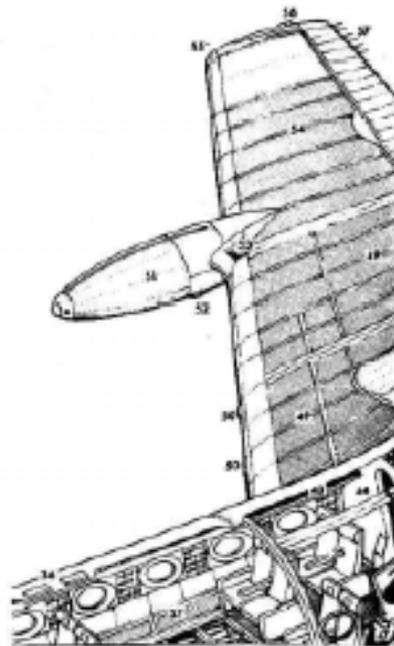
Photograph shows the spoilers (50) near the wing root.
