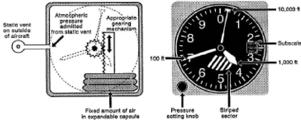
*The altimeter is a pressure-sensitive instrument.*
