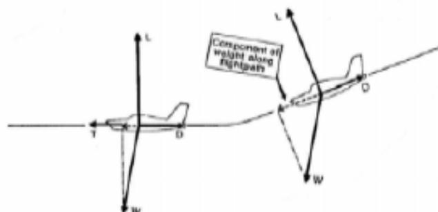
FIG 1.9. - ADDING POWER FLATTENS THE DESCENT
