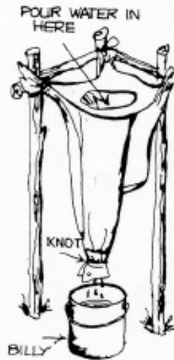
Figure 10 An Improvised Water Filter
